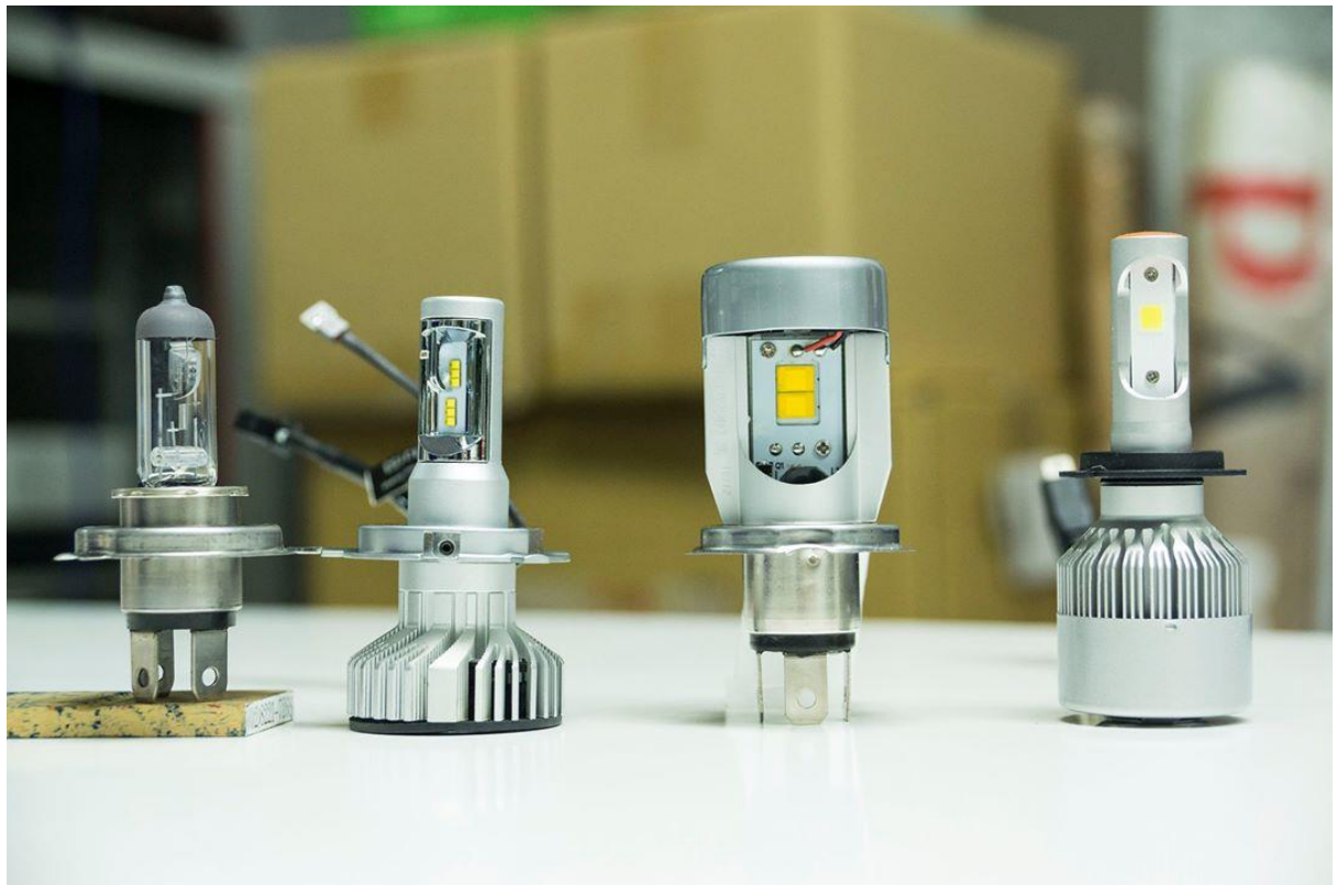
From left 1. Stock halogen 2. 11G New one 3. Old one with front Fan 4. Old Generation
